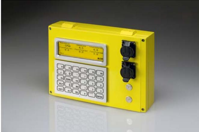
package is very compact and suitable for panel mounting or in the control cab of oilfield trucks.
