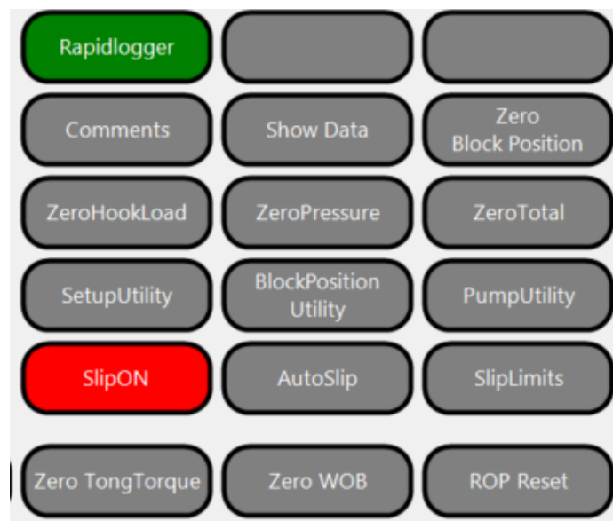
Figure 2: The driller's button panel. SlipON is red because the slips are set
