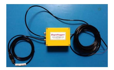
The Rapidlogger System DC-UPS power supply accepts power input from 9 to 36 Volts DC. This make it is possible to connect it directly to both 12 and 24 Volt battery type truck electrical systems.
