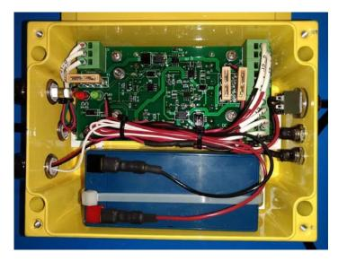
The DC-UPS contains a DC-DC power converter board, battery charging circuitry and a failover circuit to switch to backup battery power. The DC-UPS takes in dirty 9-36V DC and outputs a clean regulated constant 24VDC. Even if the input power is interrupted the output remain on until the battery drains.
