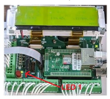
If this LED (LED1) is not lit up then there is no power being supplied to the unit and the power supply may have a problem.
