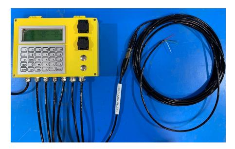
The picture above shows the outside of the Rapidlogger with the shutdown / Auxiliary cable connection.
