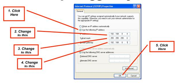
Figure 5: Internet Protocol (TCP/IP) Properties
