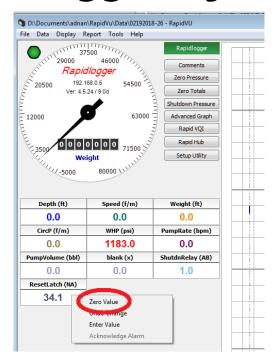
Once the relay is triggered the state is latched. In order to reset the relay the user would have to left click on the ResetLatch Variable in RapidVu and click on Zero Value.
