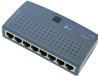
Figure 1: Network hub OR switch
