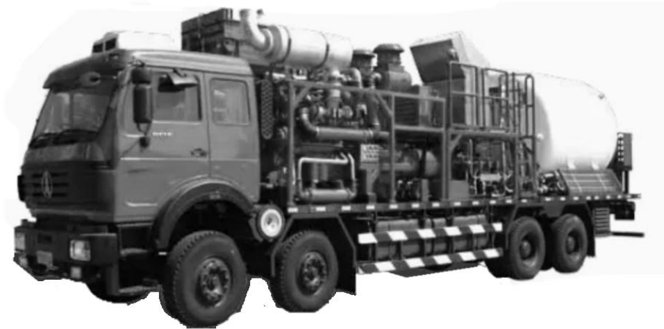
Figure 1: Nitrogen pumping unit: tank, cryogenic triplex pump, heat exchanger
